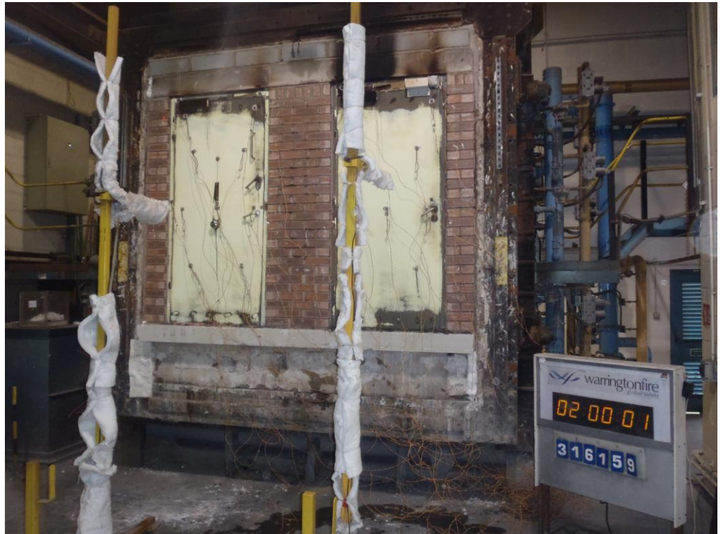
The unexposed face of the doorsets after 120 minutes of testing
