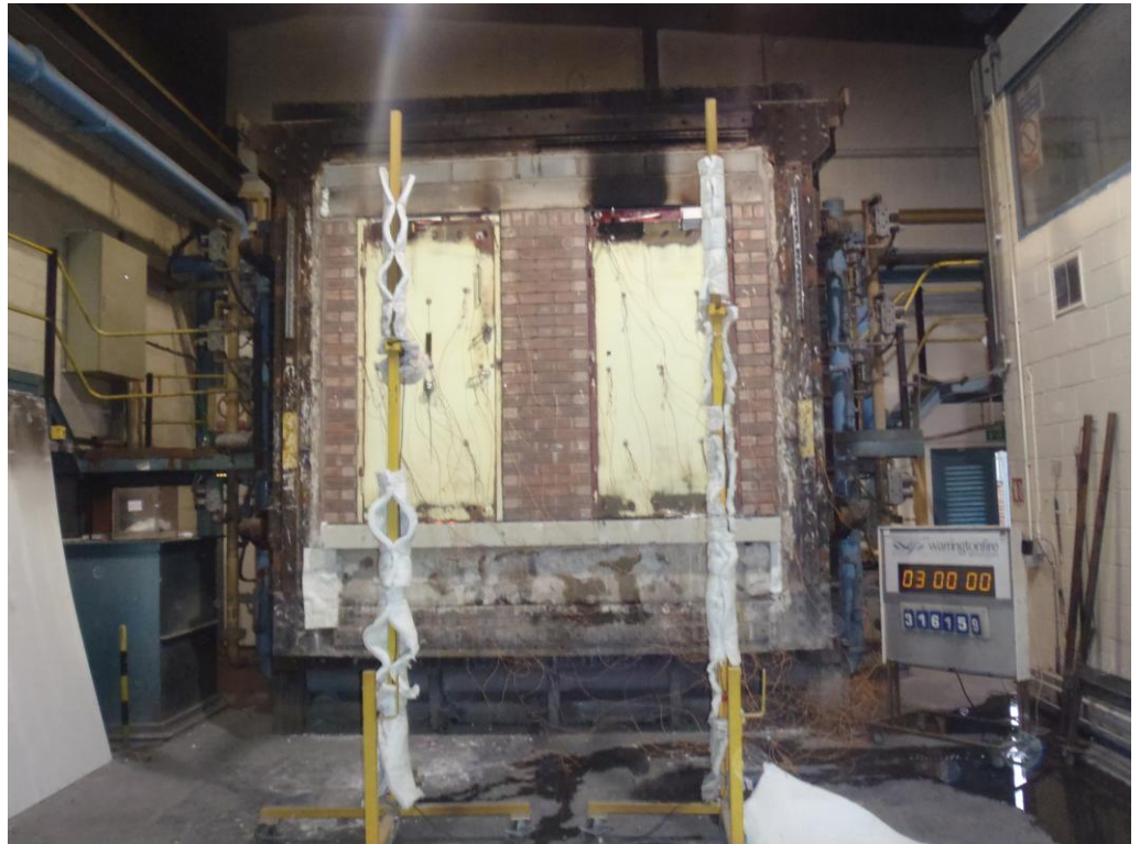
The unexposed face of the doorsets after 180 minutes of testing
