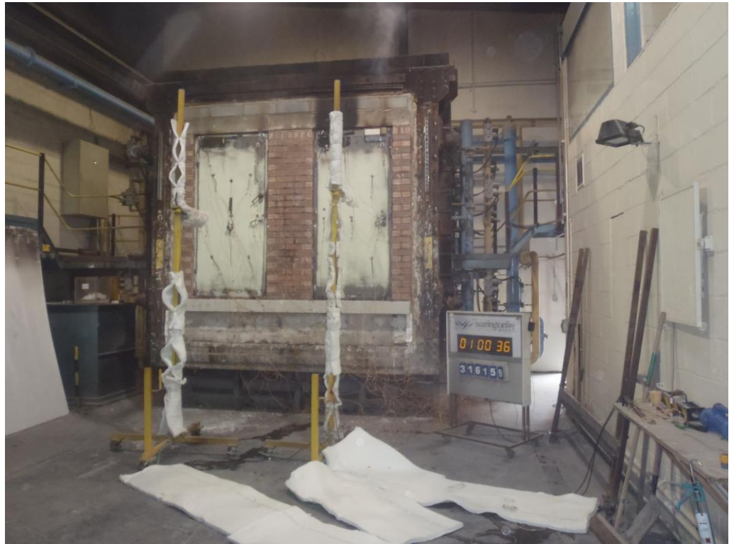
The unexposed face of the doorsets after 60 minutes of testing
