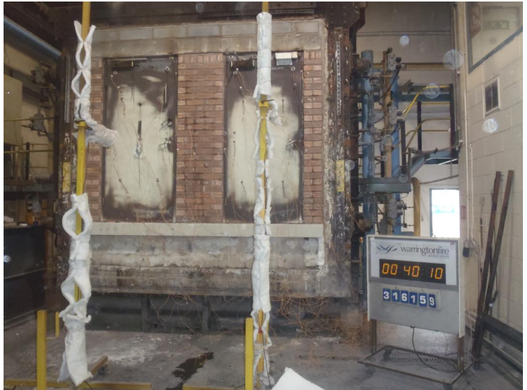
The unexposed face of the doorsets after 40 minutes of testing
