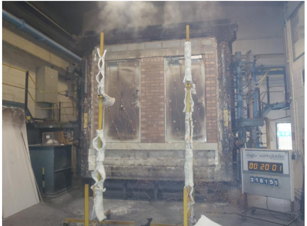
The unexposed face of the doorsets after 20 minutes of testing
