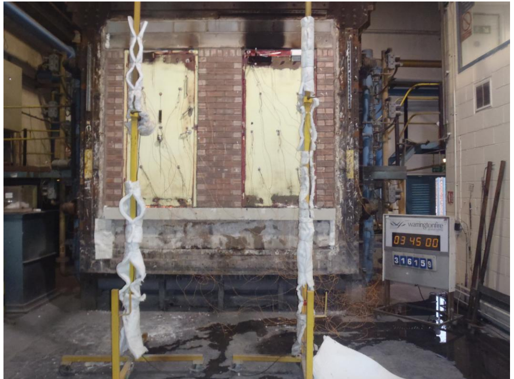
The unexposed face of the doorsets after 225 minutes of testing
