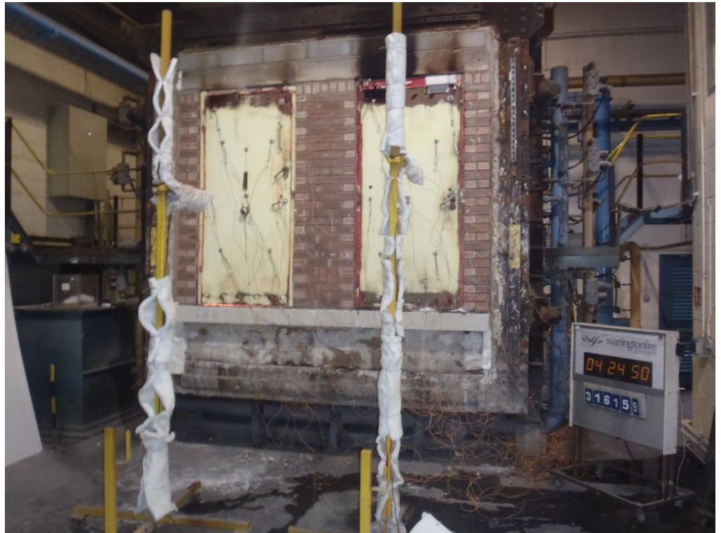
The unexposed face of the doorsets after 259 minutes of testing
