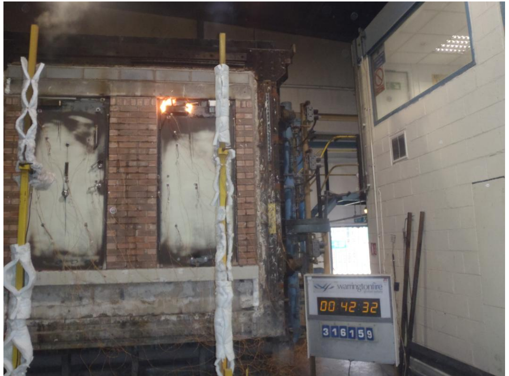
The unexposed face of the doorsets after 42 minutes of testing
