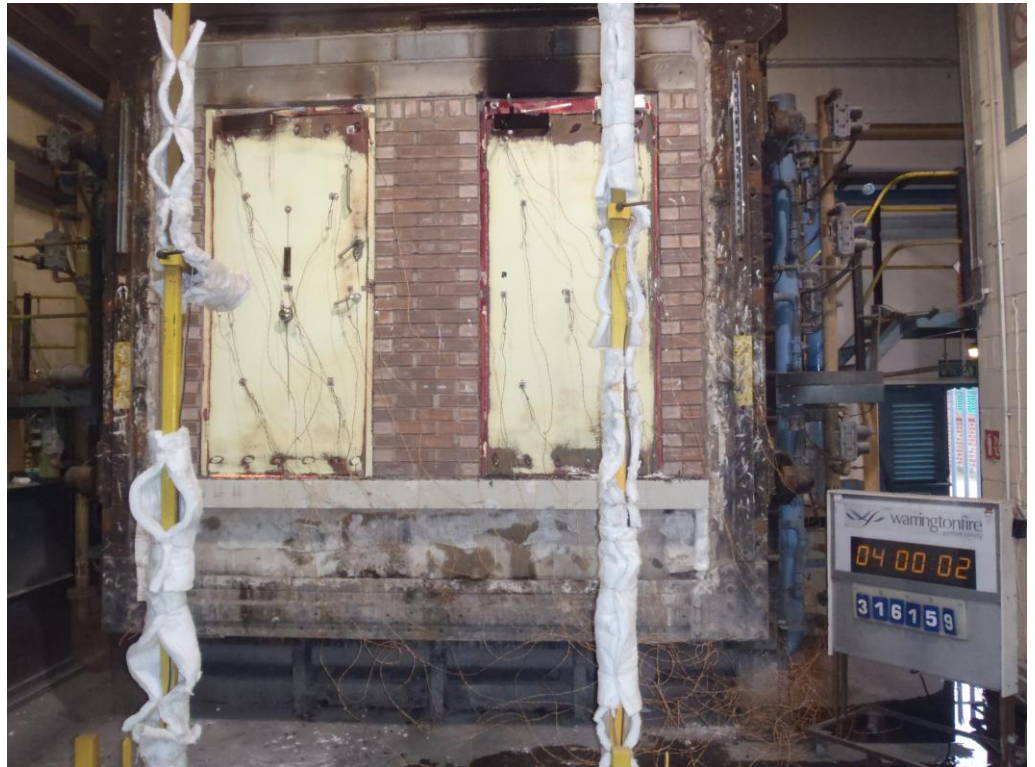
The unexposed face of the doorsets after 240 minutes of testing
