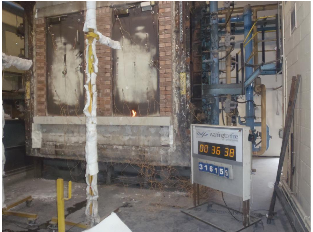
The unexposed face of the doorsets after 36 minutes of testing
